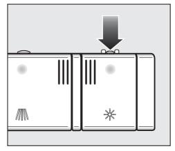
■ Press the button on the lid of the rinse aid reservoir in the direction of the arrow until the flap springs open.
